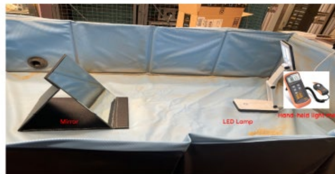
Figure 1.1 Experiment set-up showing the mirror, lamp, and light meter used.
